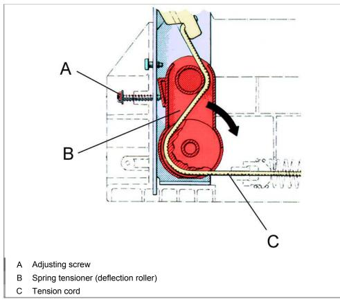
The door springs are situated on the right and left under the base pan. The tensile force is transferred to the door hinge with a tension cord (C) via a deflection roller (B). The clamping force of the spring can be increased with the enclosed adjusting screw (A) (built-in appliances only) via the deflection roller (B). If the furniture doors are very heavy (e.g.: marble), the tensile force of the standard installed springs and maximum pretension of the spring tensioner is no longer adequate.
