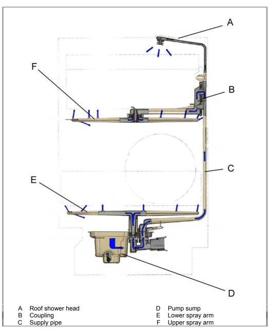
The rotor spray system consists of three spray levels, the lower spray arm (E), the upper spray arm (F) and the roof shower head (A). Water is supplied to the upper spray arm (F) and the roof shower head (A) via the supply pipe (C) attached to the inside of the tank rear panel. This pipe is connected by a direct plug-and-socket connection to one of the two outlets on the instantaneous water heater situated under the pump sump (D).
