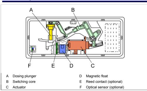
The release mechanism is activated by an actuator (C). When the actuator is actuated for the first time, the detergent-dispenser cover is opened. At the same time the release pawl engages with the switching core (B) of the rinse-aid lever so that when the actuator (C) is activated again, the dosing plunger (A) is lifted off the rinse aid.
