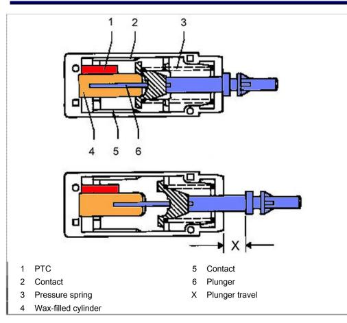
The thermohydraulic system consists of a metal cylinder with plunger. The cylinder is filled with a substance which expands greatly when heated. The heat source is a PTC (positive temperature coefficient) (1) which is in direct contact with the metal cylinder (4). A strong pressure spring (3) returns the plunger (6) back to its original position when the heat source is switched off.
