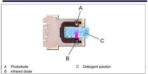
The infrared light-emitting diode (B) and the photodiode (A) are located opposite each other in a U-shaped translucent housing on a board.
