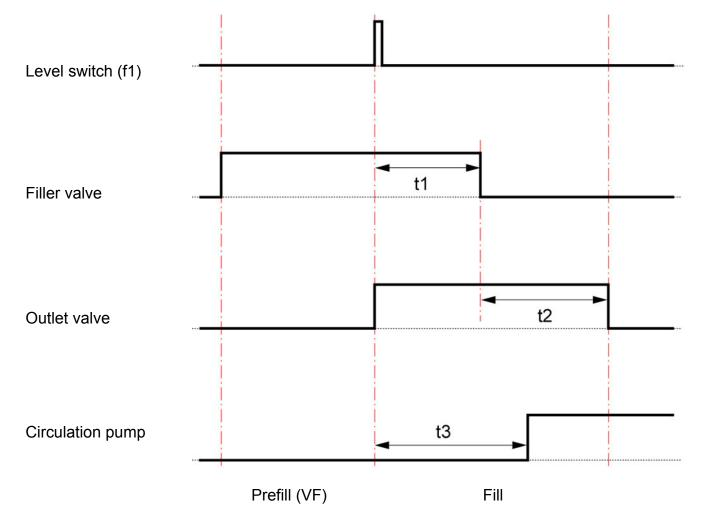
t1 = calculated refill time, t2 = run-on time of drainage valve, t3 = switch-on delay of circulation pump
