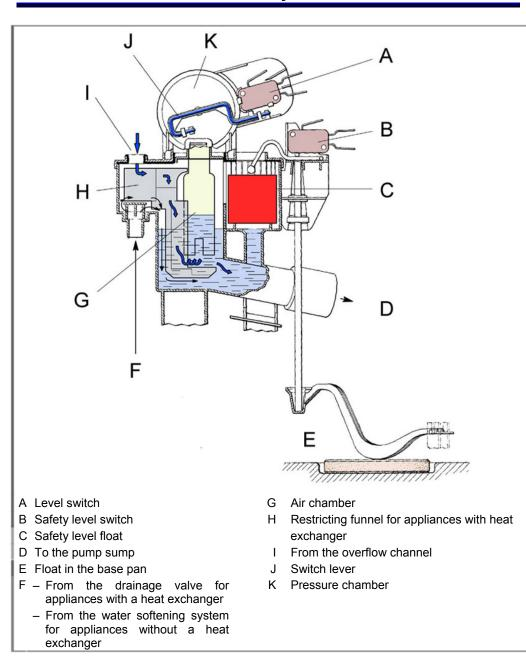
If the dishwasher controller or components malfunction, causing the machine to overfill, the valve combination is closed via the safety system, shutting off the water supply.
