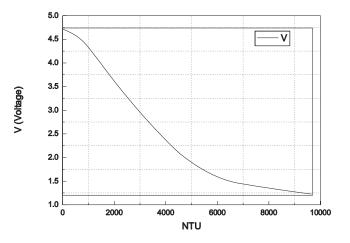
Application Section Detecting the turbidity degree of water
